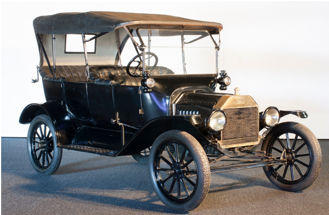
Photo: This 22 hp, 4-cylinder Model T Tourer was made at Ford's Walkerville factory, Ontario, Canada, in 1916. Ford Canada supplied cars to the British Empire. MAAS collection, B727-1
