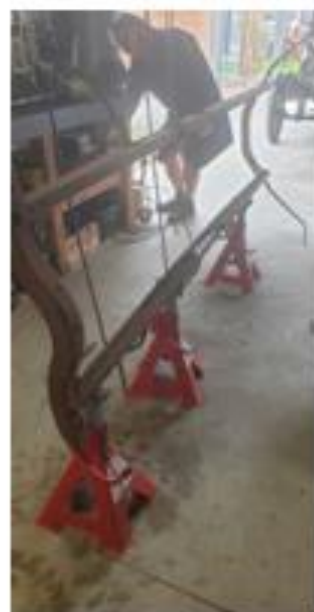
Hot riveting the replacement chassis
