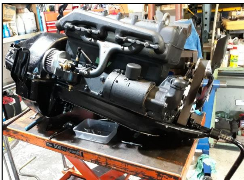
Fully rebuilt engine and transmission ready for installation
