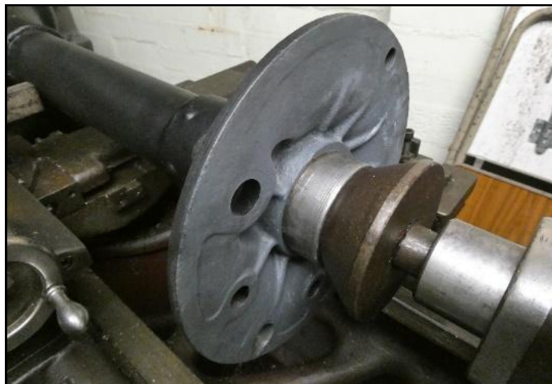
Live centre in the outer housing bearing opening, sitting right up on the taper ready to spin and check for straightness.
