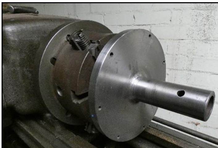
This is the fixture that holds a standard axle housing. The axle housing bolts to the flange and the extension slides inside where the bearing sleeve would normally be.
