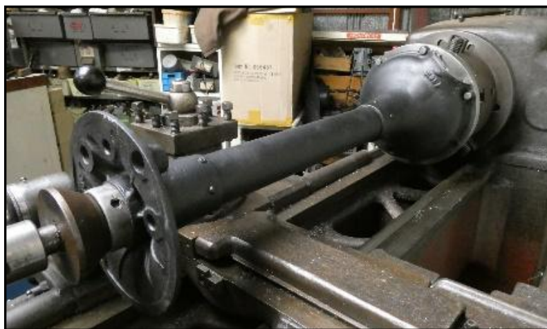
Live centre in the outer housing bearing opening, sitting right up on the taper ready to spin and check for straightness.
