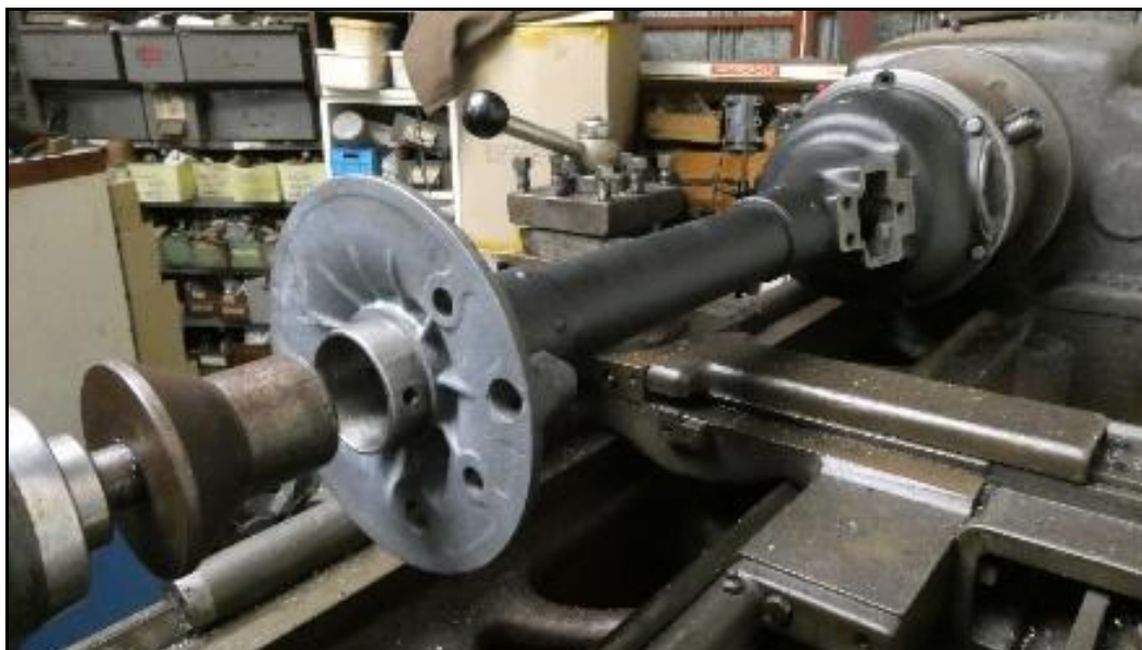
Standard housing and Ruxstell housing set up in the jig, checking for straight.
