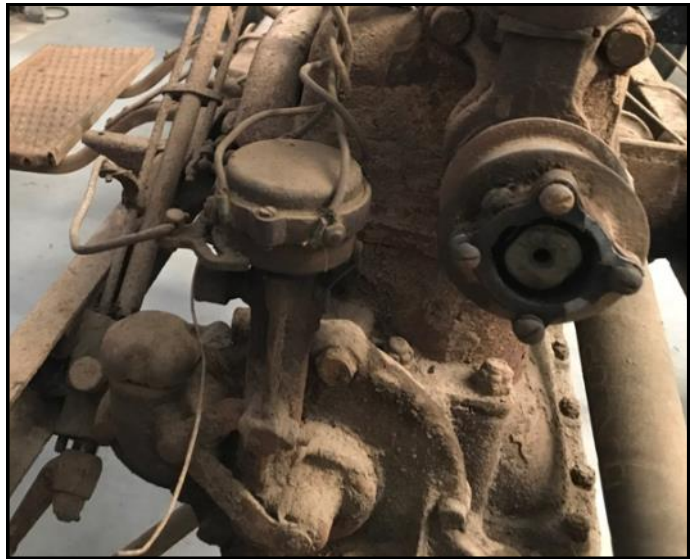
Original accessory Riser Timer replaced with more standard type Anderson cam mounted timer.
