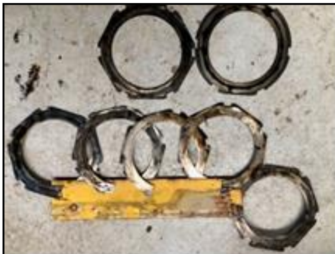
Worn out clutch plates
