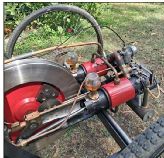
Above Left: Flywheel, cylinders and oilers
