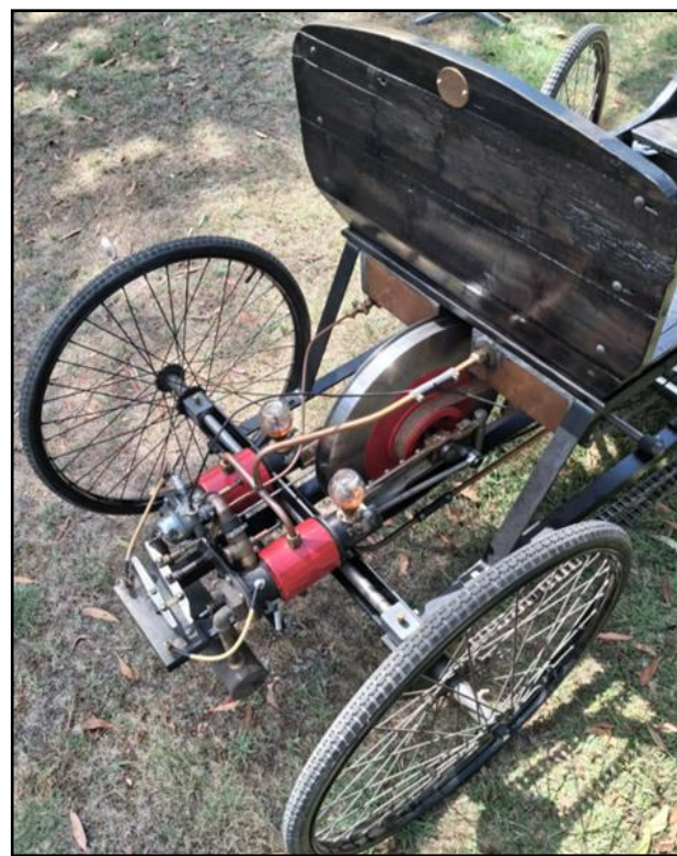
Above Left: Flywheel, cylinders and oilers
